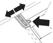
Open latch lever of righthand tractor. Align it to paper width. Insert fanfold paper into tractor. Make sure it is inserted by the same length as on left-hand tractor to avoid paper jam. Close flap and lock by turning lever to the rear.
